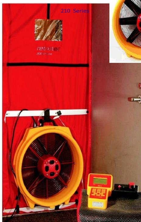
It is common practice in the offshore industry to pressurise TR's to between 50 and 75 Pa. to measure pressure decay against time. From this an air leakage rate is calculated and used as a performance measure of the structure's integrity.
