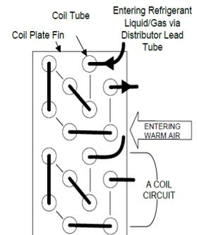
Some evaporator coils do not have a distributor, on this type of coil; correct sizing of the headers, lead tubes, coil circuiting, size, fin surface type and FPI are even MORE critical. Once this type of evaporator is built, the pressure drop through this coil can not be adjusted, unlike the variants with a nozzle where changes can be generated to achieve the desired overall pressure drop.
